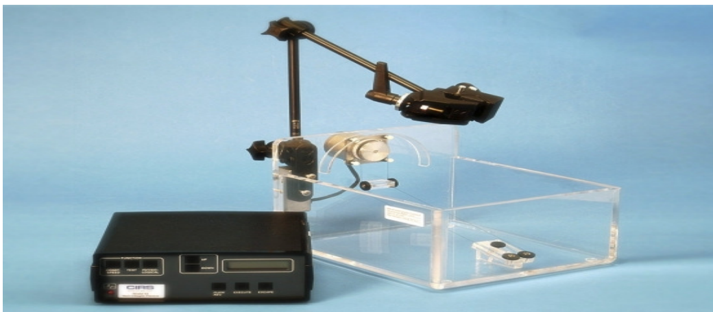
Figure 4.5 Components of a moving string phantom
